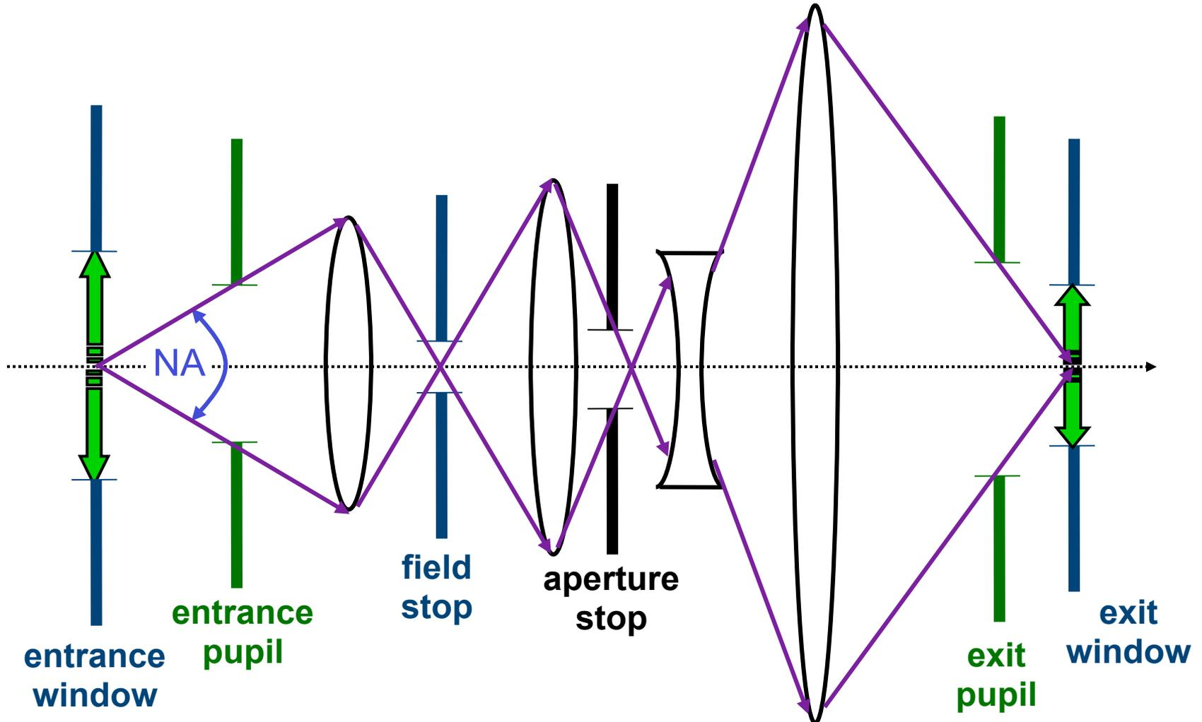
The Numerical Aperture is the angle between the pair of Marginal Rays that just make it through the edges of the Aperture Stop
