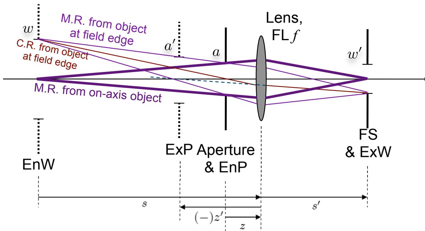
**Note:** The angular acceptance of rays emanating from an off-axis point object is *smaller* than the angular acceptance of rays from an on-axis point object.
