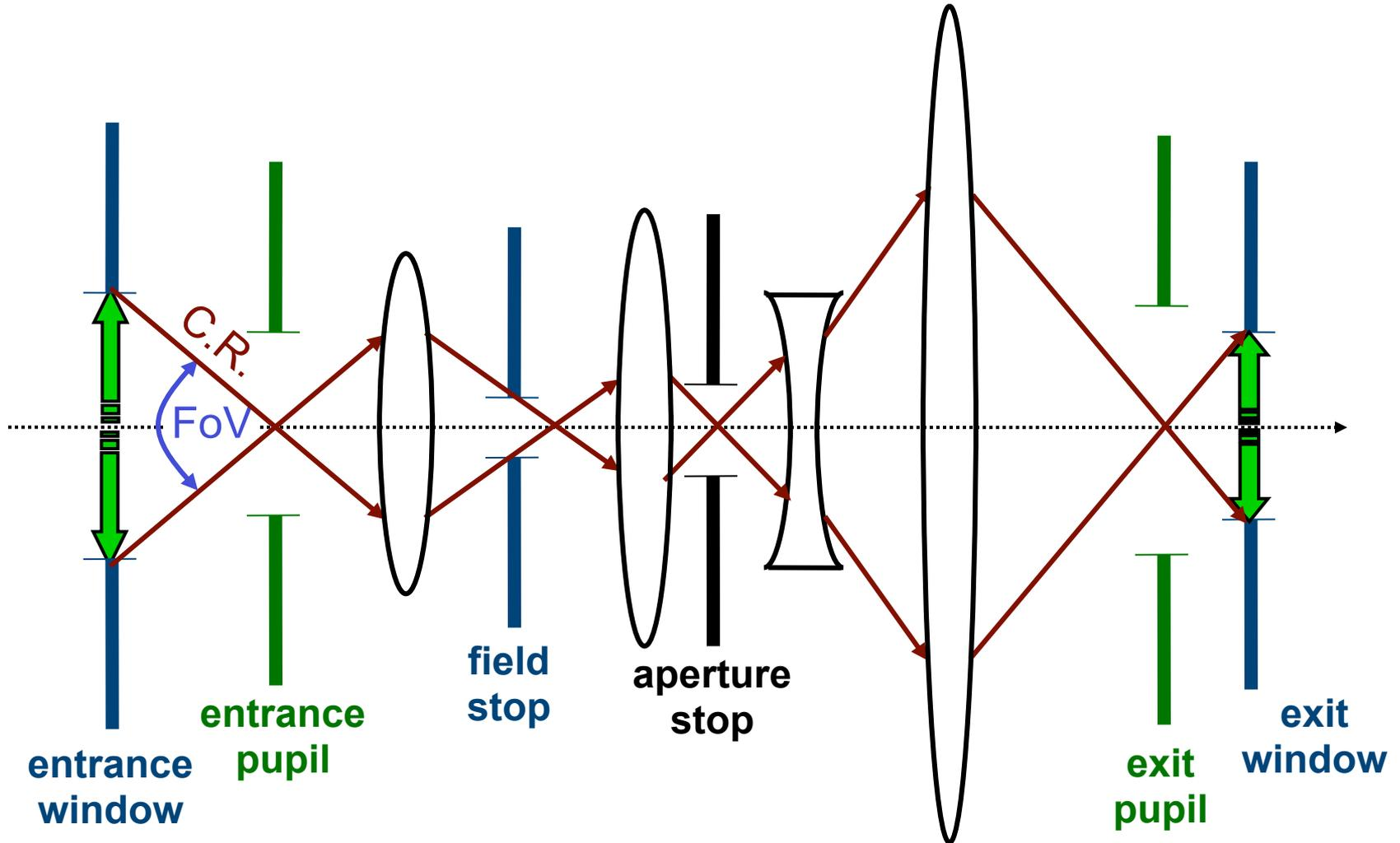
The Field of View is the angle between the pair of Chief Rays that just make it through the edges of the Field Stop
