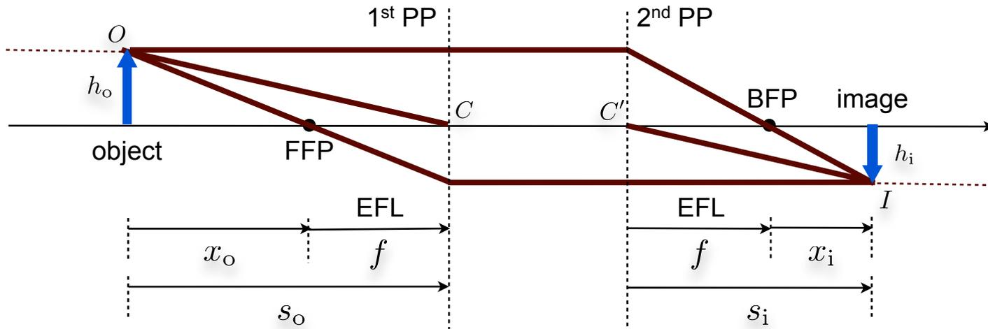
$$x_o x_i = f^2; \quad \frac{1}{s_o} + \frac{1}{s_i} = \frac{1}{f}; \quad M_T = -\frac{x_i}{f} = -\frac{f}{x_o} = -\frac{s_i}{s_o}; \quad M_A = \frac{1}{M_T}.$$
