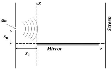
In our problem, let's assume the mirror is placed at the plane x = 0 and illuminated by a spherical wave originating from the slit at location  $(x_0, -z_0)$  (where  $x_0, z_0 > 0$ ). Using the paraxial approximation for a 1D spherical wave (y=0),
