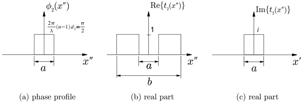
Figure 2: complex transparency of the grating  $T_2(x'')$
