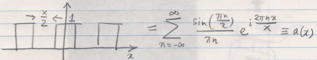
The diagram shows a grating with period  $X$  and a central slit of width  $\frac{X}{2}$ . The Fourier transform integral is given by:
