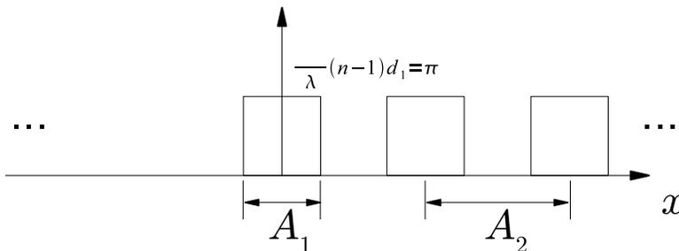
Figure 1: phase profile of the grating  $T_1(x)$
