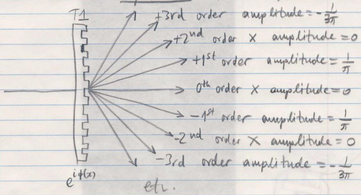
Lens L1 focuses each diffracted order to a focal point just before T2:
