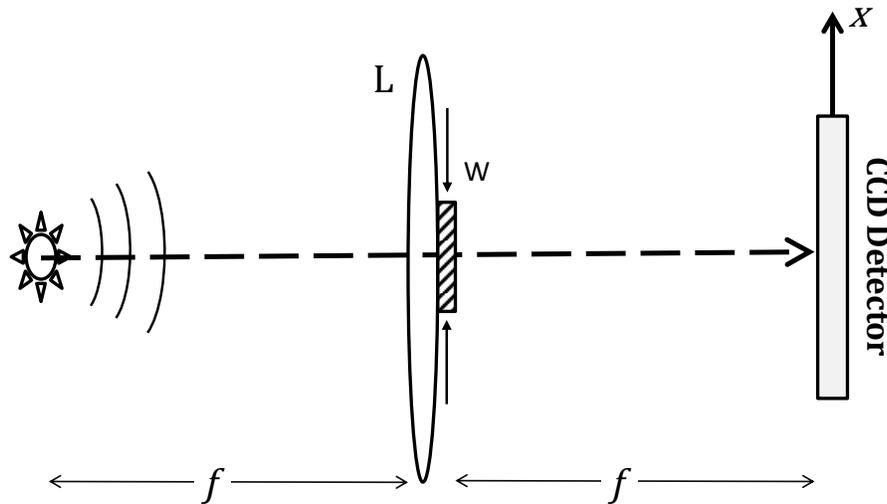
Let's assume the lens is placed at the plane  $z = 0$  and illuminated by a spherical wave originating on-axis at location  $z = -f$  (where  $f > 0$ .) Using the paraxial approximation for the spherical wave ( $y=0$ ),
