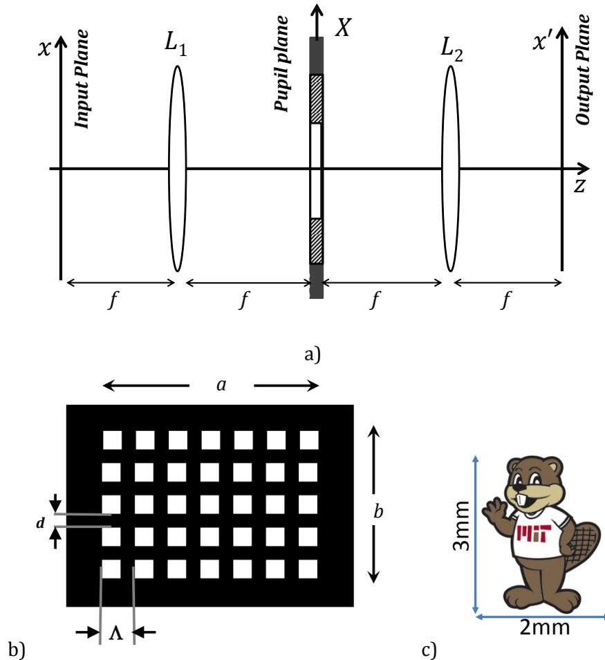
Figure 2. 4F imaging system with a square mesh grid as amplitude mask (dark area is completely opaque, and white area is transparent) placed at pupil plane( $X, Y$ ).
