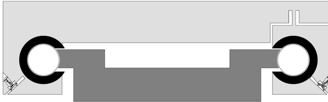
Flexure that is stiff in y and z, yet compliant in x
