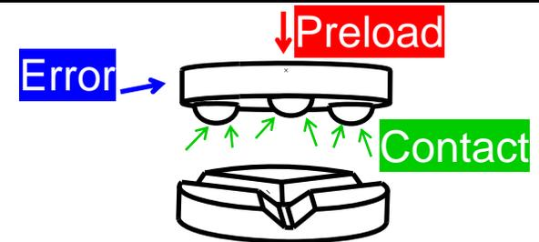
$$\Sigma \vec{F}_{relative} = 0 = (\vec{F}_{preload} + \vec{F}_{Error}) + (\vec{F}_{Ball\_1} + \vec{F}_{Ball\_2} + \vec{F}_{Ball\_3} + \vec{F}_{Ball\_4} + \vec{F}_{Ball\_5} + \vec{F}_{Ball\_6})$$
