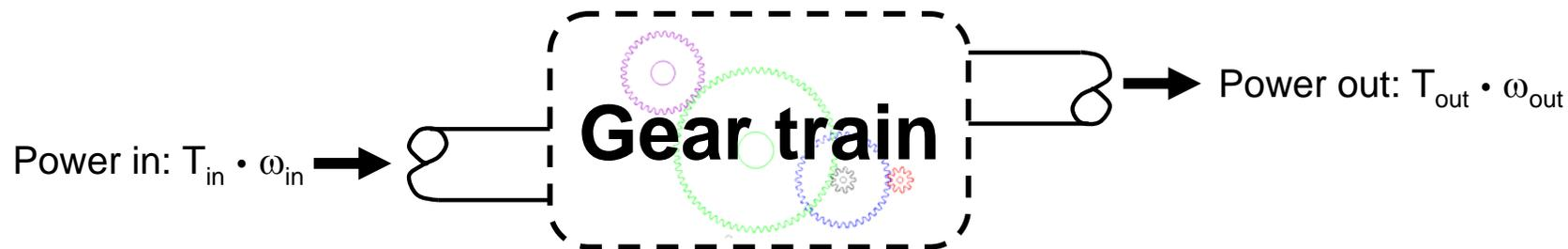
Transmission ratio for elements in series:  $TR = (\text{proper sign}) \cdot \frac{\omega_{out}}{\omega_{in}}$
