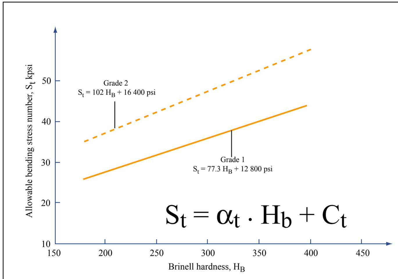
Figure by MIT OpenCourseWare. Adapted from Fig. 14-2 in Shigley & Mischke.
