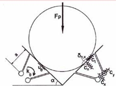
Ball in V-Groove with Elastic Hinges
