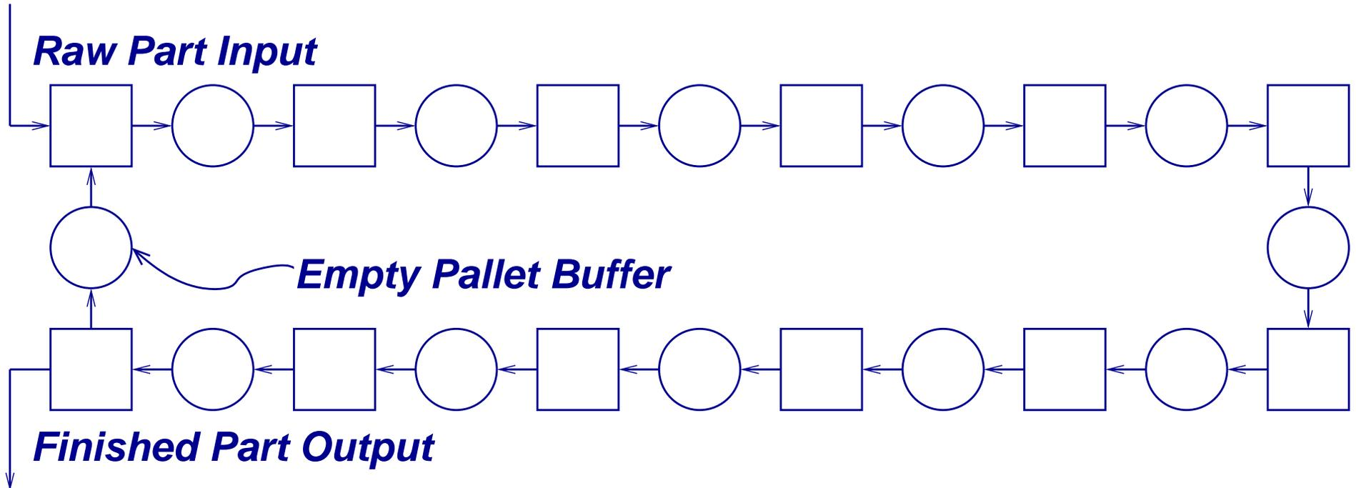
Pallets or fixtures travel in a closed loop. Routes are determined.
