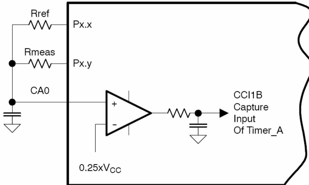
Result only dependent on the ratios of the test and reference resistors
