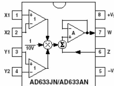
8-Lead Plastic SOIC (RN-8) Package
