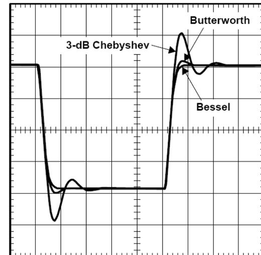
Figure 11. Transient Response of the Three Filters
