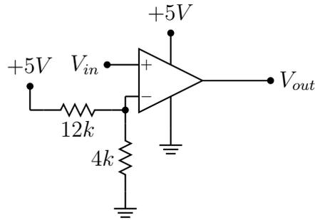
Figure 3: Comparator circuit.
