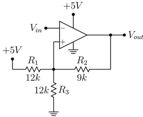
Figure 5: Schmitt triggered input design for problem 3.
