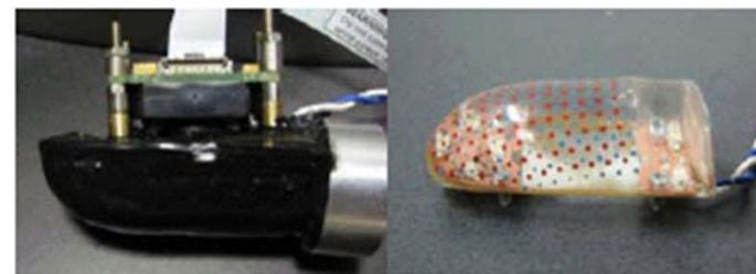
Figure 10: Endowing an robotic finger with the sense of touch
