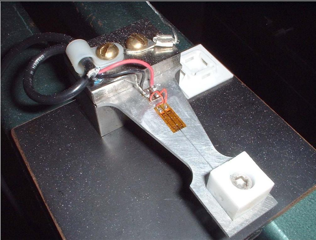
*Simple, “naked” load cell from Ohio State*
