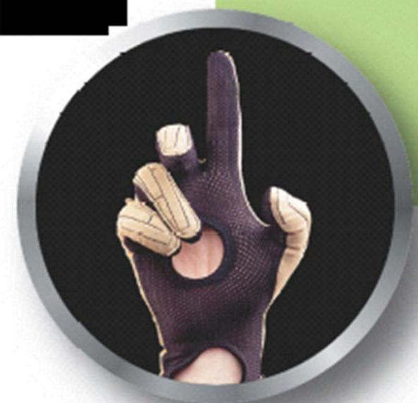
The 22-sensor CyberGlove has three flexion sensors per finger, four abduction sensors, a palm-arch sensor, and sensors to measure flexion and abduction. Each sensor is extremely thin and flexible being virtually undetectable in the lightweight elastic glove.
