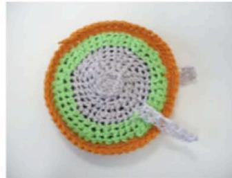
Here is the crochet pressure sensor. The main principle is same as regular pressure sensor. Instead of conductive fabric or thread, I used conductive yarn from Schoeller, Nm 50/2 60/40 Pes/Inox @ Euros 65.00/kg (25,000 metres/kg). Since this yarn is very thin, it is mixed with normal yarn and crochet, which is what you can see [...]
