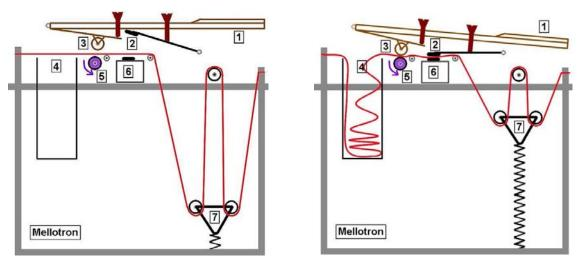
The Mellotron spools the tape prior to the key being pressed (left). When the key is pressed, the tape head clamps down on the tape, and its content is played (right). When the key is released, the spring pulls the tape back into place.<sup>3</sup>
