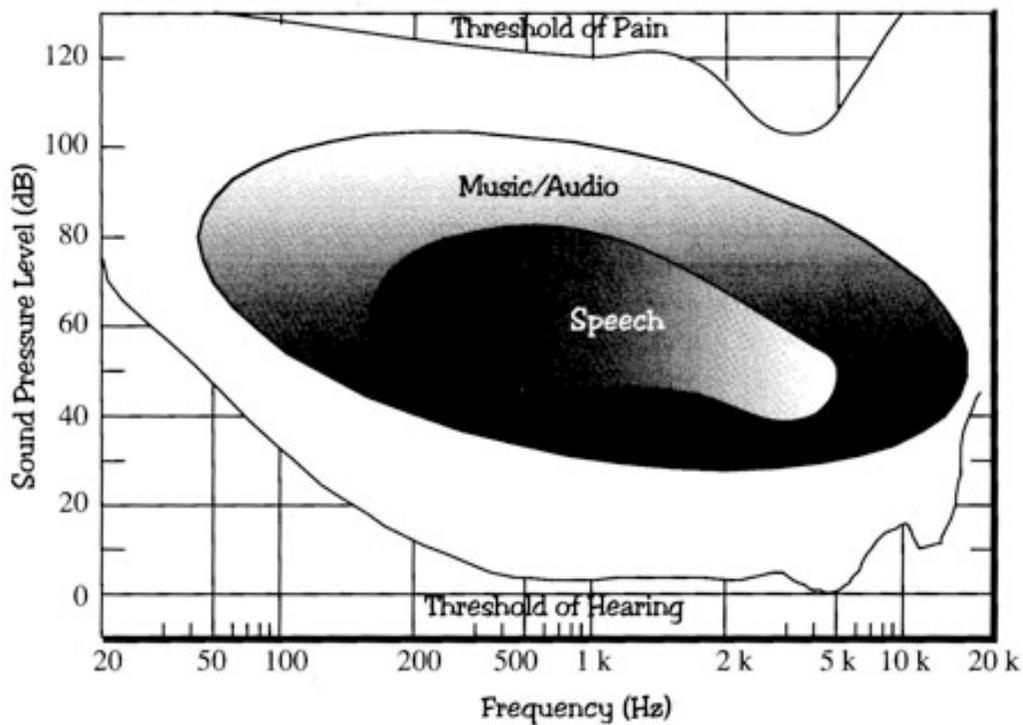
*Fig. 11.1. A more detailed picture of our audio window. Most music does not exceed a range of level of about 75 dB from softest to loudest. Similarly, most recorded music does not contain much information above 18 kHz.*
