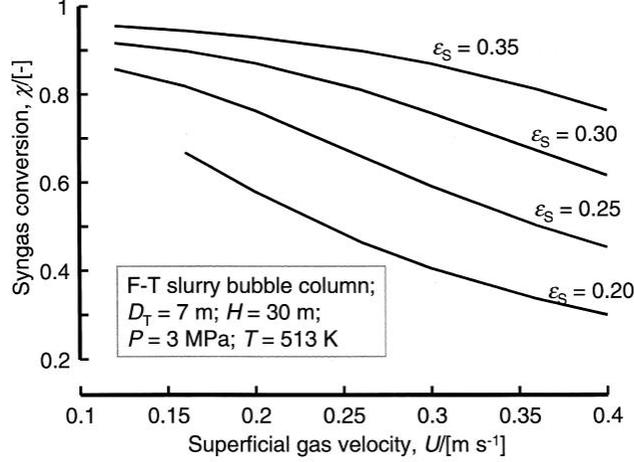
Figure 3: Effect of catalyst concentration on conversion ratio
