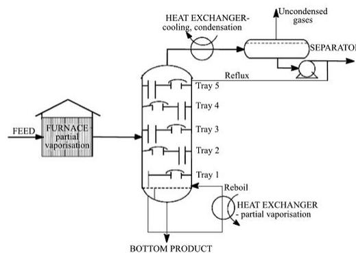
Figure 9: Distillation unit
