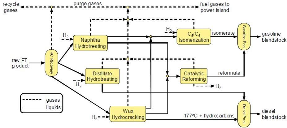
Figure 10: Schematic of FTL refining process
