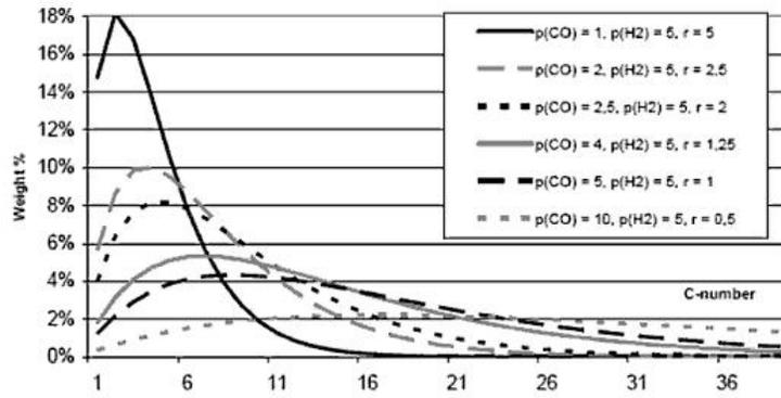
Figure 6: The effect of feed ratio  $r = H_2/CO$  on selectivity at  $T=300^\circ C$
