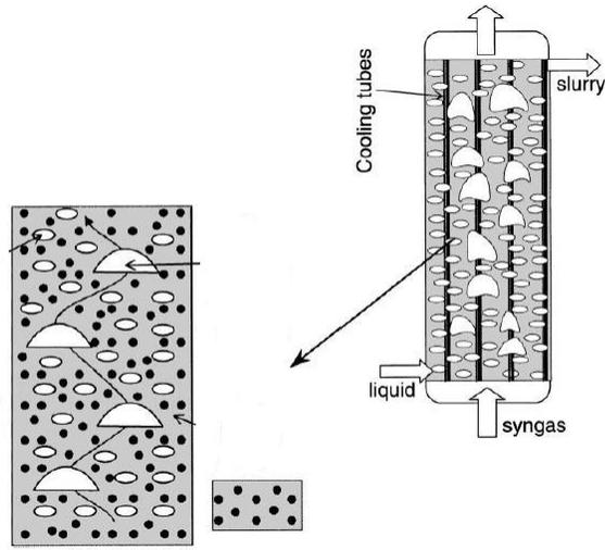
Figure 1: Slurry phase bubble reactor schematic [1]
