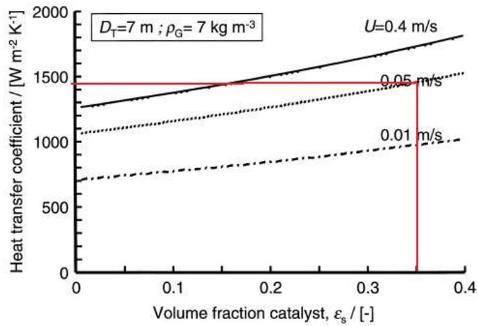
Figure 7: Heat transfer coefficient as a function of catalyst concentration
