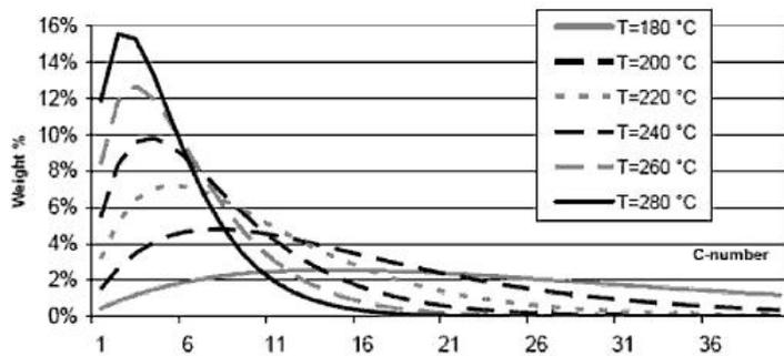
Figure 5: The effect of temperature on selectivity at  $H_2/CO = 2.0$
