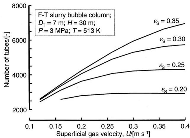
Figure 4: Effect of superficial velocity, catalyst concentration on the number of coolant tubes R. Krishna [2]
