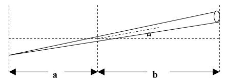
The solid angle is proportional  $to cos^2(\theta)$ . The angle between rays and detector is proportional  $to cos(\theta)$ . The effective spot size of the hole is proportional  $to cos(\theta)$ . Therefore, I is proportional to  $cos^4(\theta)$ .
