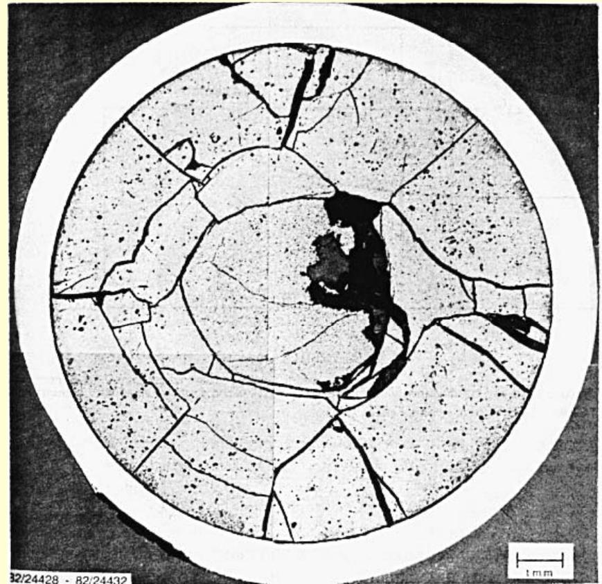
Example of a Cracked Fuel Cross Section
