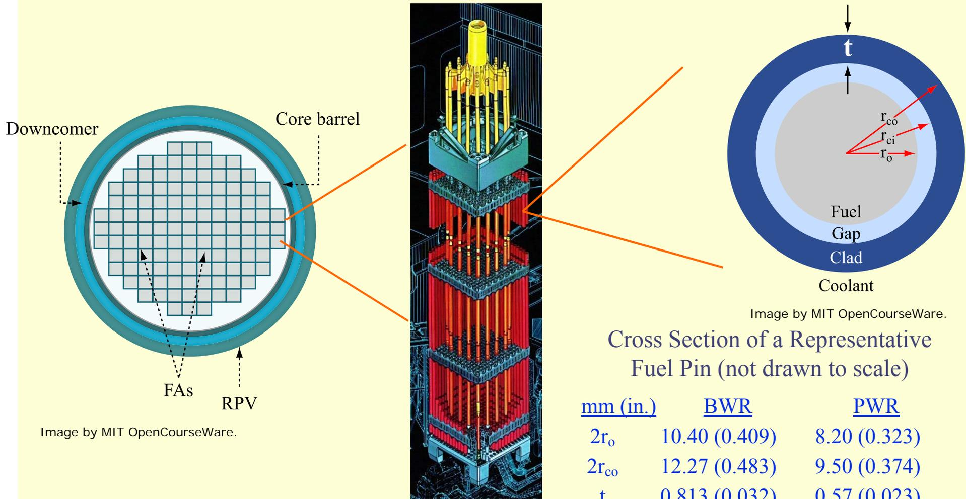
Cross Section of a Representative Fuel Pin (not drawn to scale)
