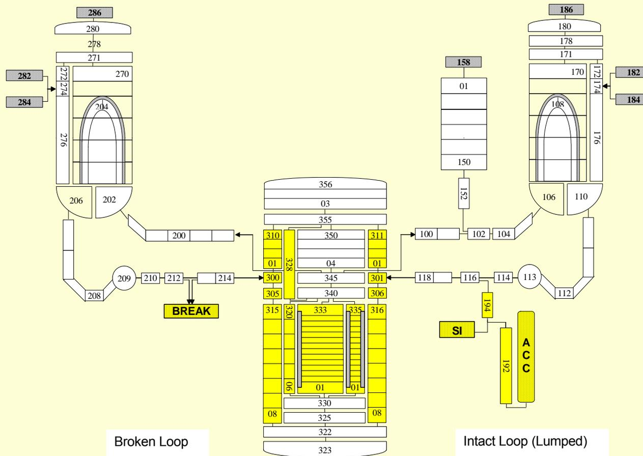
3 intact loops are lumped into one with functioning LPCI train
