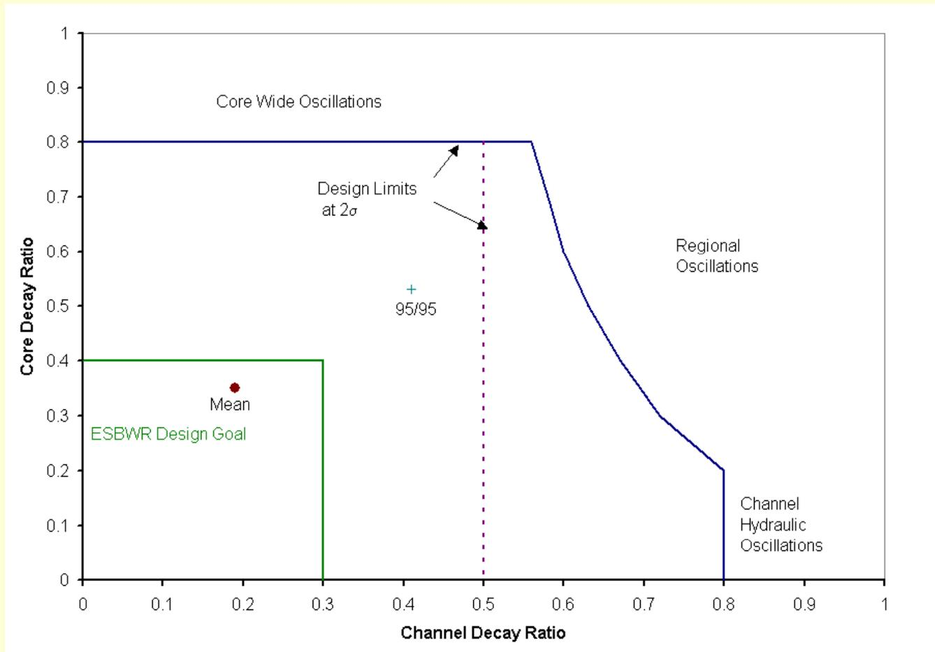
ESBWR is designed to operate with significant margin to any instability regions
