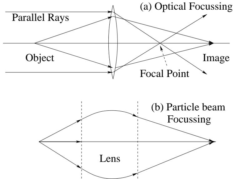
Figure 2.4: Analogy between optical and particle-beam focussing.
