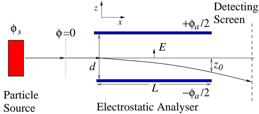
Figure 2.2: Schematic of electrostatic acceleration and analysis.
