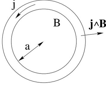
Figure 3.3: Force on a solenoid magnet.
