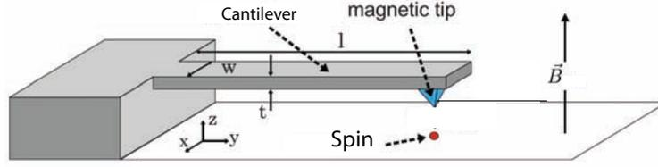
Figure 1: A cantilever coupled to a spin. Adapted from P. Rabl, P. Cappellaro, M.V. Gurudev Dutt, L. Jiang, J.R. Maze, and M.D. Lukin, “Strong magnetic coupling between an electronic spin qubit and a mechanical resonator”, Phys. Rev. B 79, 041302 R 02 (2009)
