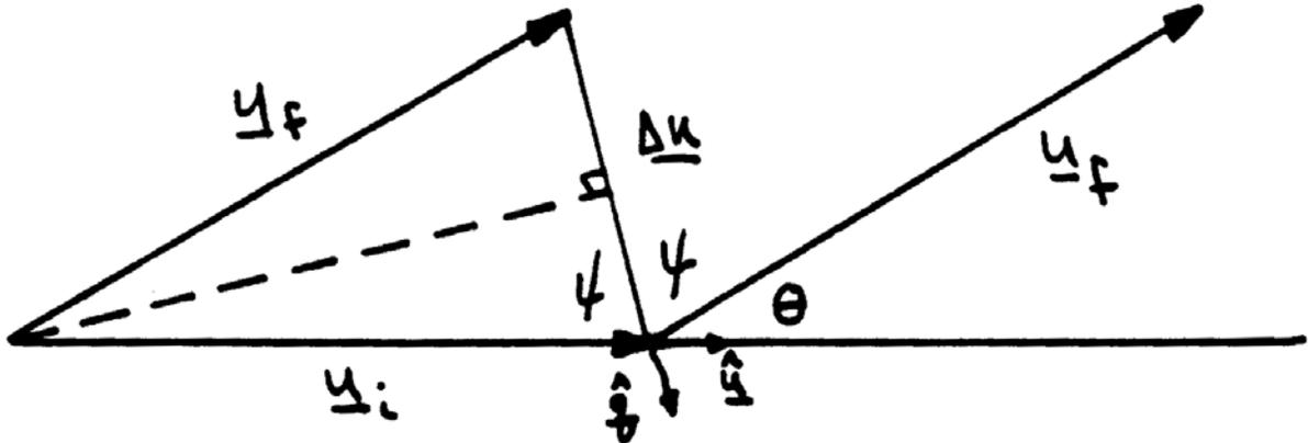
Geometry of the scattering event showing relative velocities before,  $\mathbf{u}_i$ , and after,  $\mathbf{u}_f$ , the collision.
