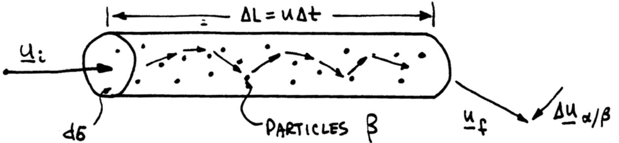
Schematic of test particle  $a$  scattering from a distribution of field particles,  $b$ .
