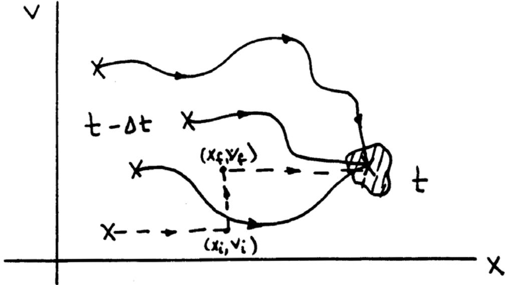
Evolution of phase space with scattering present. Arrows depict possible paths. The dotted path suggests the route followed by a particle undergoing a collision between  $t - \Delta t$  and  $t$ .
