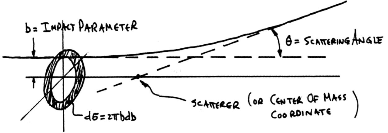
Collision in center of mass frame showing trajectory of relative coordinate.
