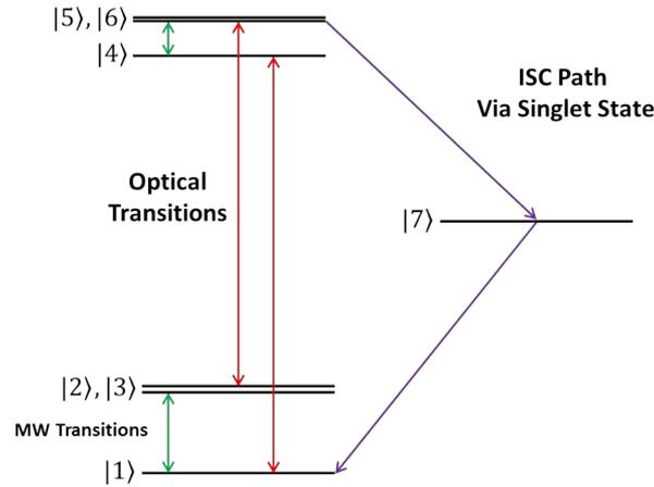
**Figure 1:** The seven level model in the absence of an external magnetic field, consisting of the ground state and excited state triplets and a metastable singlet. Only spin-conserving radiative transitions and non-radiative transitions to the metastable state are considered.
