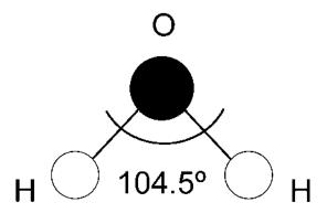
The water molecule,  $H_2O$ , is composed of 2 atoms of hydrogen (molecular weight 1 amu =  $1.66 \times 10^{-27}$  kg) each bonded to one atom of oxygen (molecular weight 16 amu) in a triangular arrangement. The oxygen-hydrogen bonds have a length  $r = 9.6 \times 10^{-11}$  m and are set apart by an angle of  $104.5^{\circ}$ . Treat each atom as a point mass.
