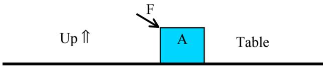
There may or may not be friction between the block and the table. Assume that the block **does not move** at all. Which of the following is true (only one is correct)?
