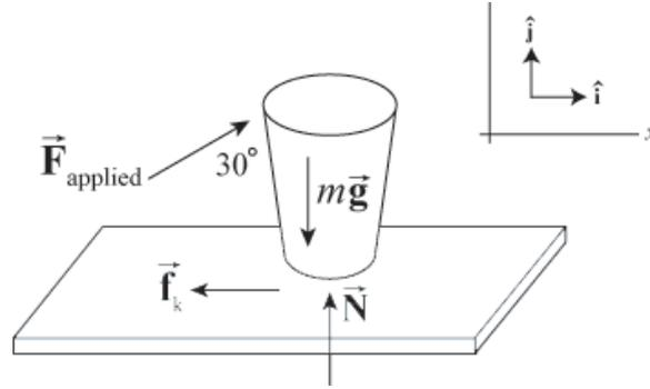
**Figure 11.3** Force diagram on cup.
