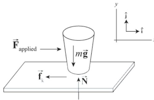
**Figure 11.2** Force diagram for cup.
