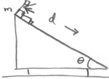
A child's playground slide is  $d = 5.0m$  in length and is at an angle of  $\theta = 2.0 \times 10^1 \text{ deg}$  with respect to the ground. A child of mass  $m_b = 2.0 \times 10^1 \text{ kg}$  starts from rest at the top of the slide. The coefficient of sliding friction for the slide is  $\mu_k = 0.2$ .
