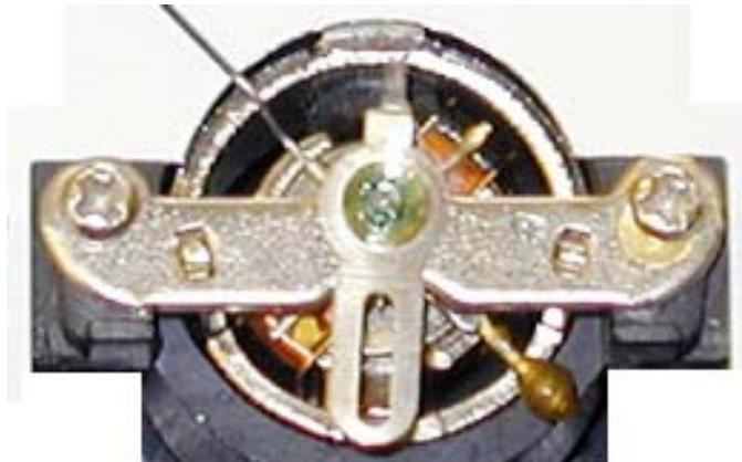
**Figure 2: Multimeter Coil**
