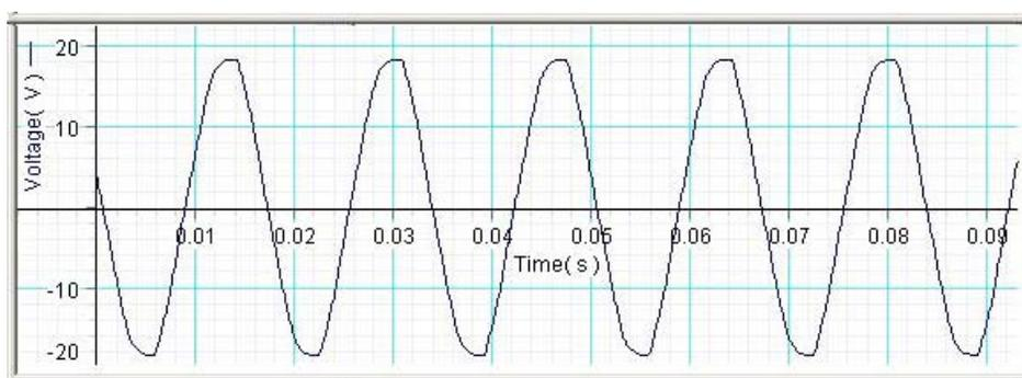
**Figure 4: Wall transformer output voltage**
