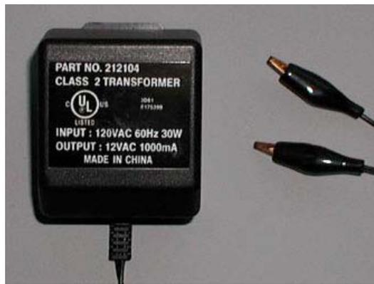
**Figure 3: Wall transformer**
