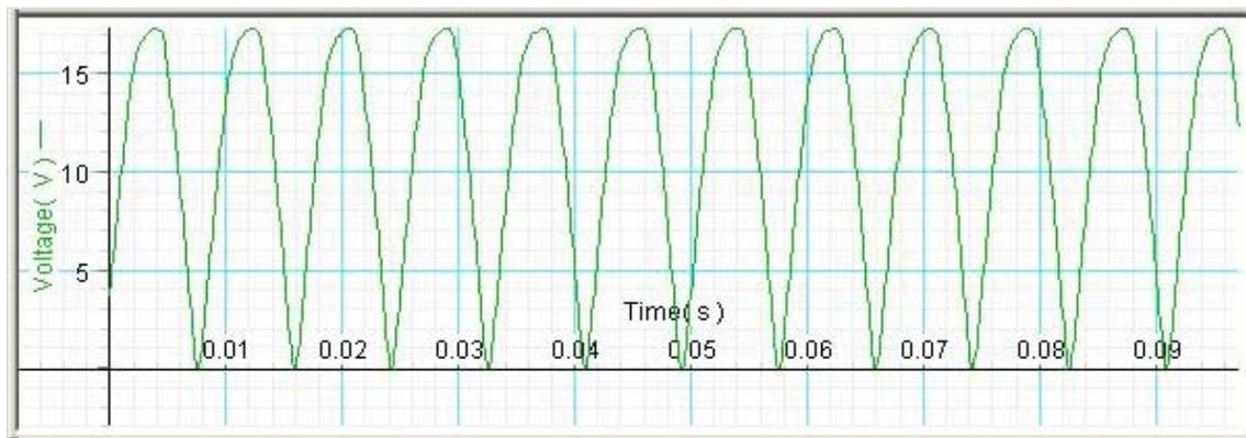
**Figure 9: Voltage output from the bridge rectifier**
