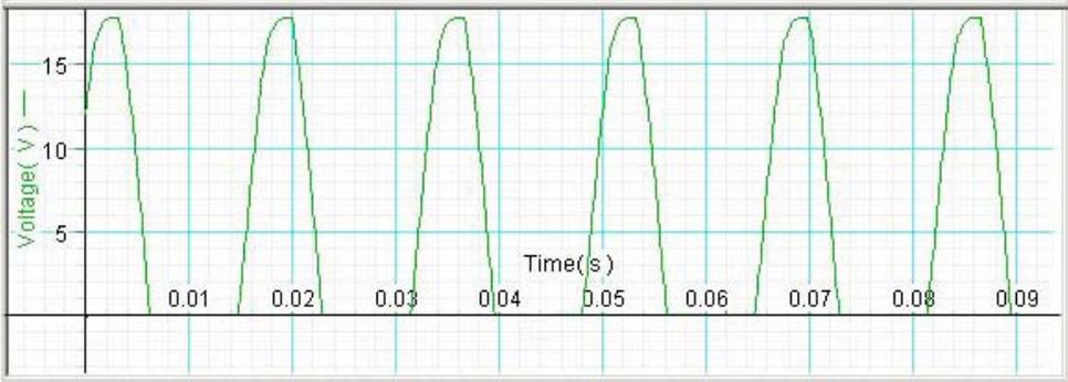
Figure 6: Rectifier sine wave after passing through half-wave rectifier
