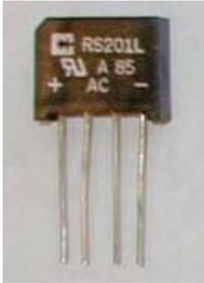
Figure 7: Bridge rectifier
