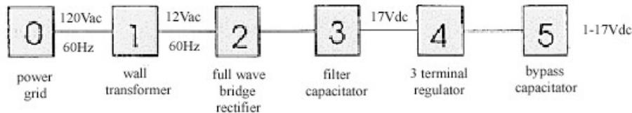
Figure 1: Block diagram of LVPS
