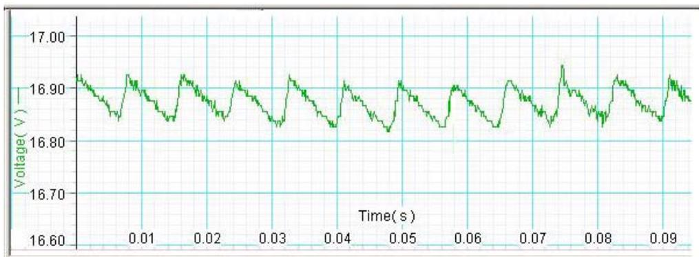
**Figure 11: Smoothed out voltage due to  $1000\mu F$**
