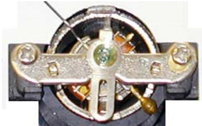
**Figure 2: Multimeter Coil**
