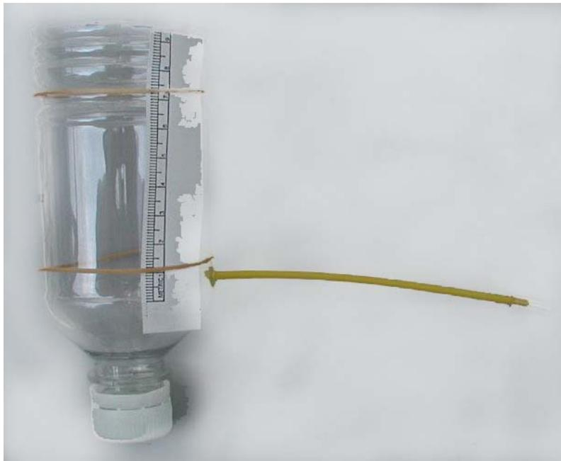
**Figure 3: Container, ruler, and stirrer inserted in hole**
