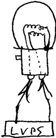
When you clip the LVPST output leads to the bottom two input leads to the light, the two filaments are in series and there is not enough power to light both filaments, so the 27W filament becomes dull red, and then dark. However the 8W filament still lights. The power is
