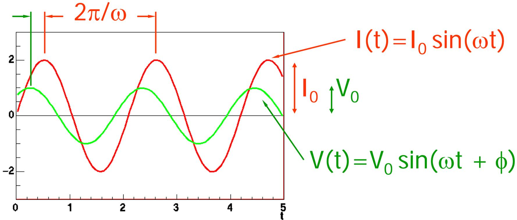
Impedance  $Z = V_0/I_0$
