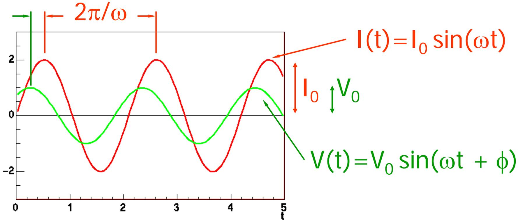
Impedance  $Z = V_0/I_0$
