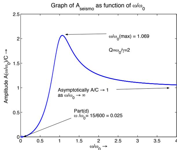
d) Period of the Seismograph  $T_s$  is 30 s and  $Q$  is 2.
