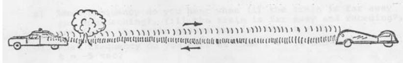
The radar transmitter is not moving. The reflected beam is again received by the police; the frequency  $f'$  of this reflected signal is measured by a stationary receiver on the police car. From this, the velocity  $v$  of the car is calculated. All this is done in a “black-box” in less than a small fraction of a second! A digital display tells the police officer your speed nicely converted into miles/hour.
