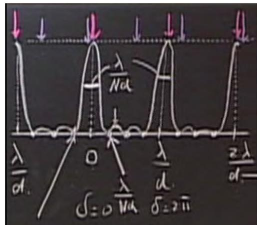
maxima are, the first peak away from  $\theta = 0$  for  $N = 4$  has an intensity  $I = 1.17I_0$ , much smaller than the  $16I_0$  of the principal peaks (21:00). The more slits, the better the spectral resolution. The
