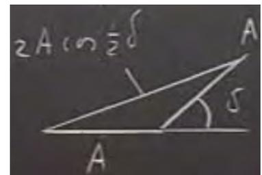
Therefore, the end angle of the small triangle is  $\delta/2$ , and with the hypotenuse length  $A$ , the 3<sup>rd</sup> side has length  $A \cos(\delta/2)$ , so the length of the long side of the big triangle is  $2A \cos(\delta/2)$ .
