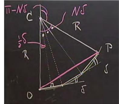
these notes)  $OP = 2R \cos((\pi - N\delta)/2)$ . Substituting for  $R$ , and using a trig identity to simplify the cosine term gives:  $OP = A \frac{\sin((N\delta)/2)}{\sin(\delta/2)}$ .
