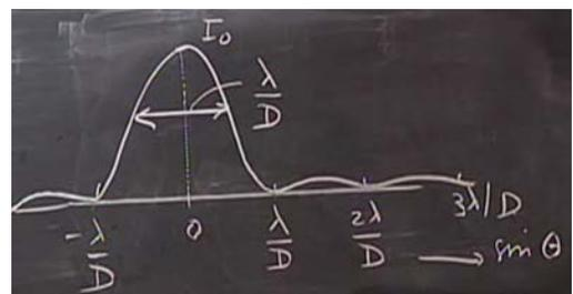
the slit is, the wider will be the pattern. The first mini-maximum, at  $\sim 1.5\lambda/D$ , has  $\beta = 1.5\pi$ ,  $\sin \beta = -1$ , and  $I = 0.045I_0$ . The maxima farther out are even smaller.
