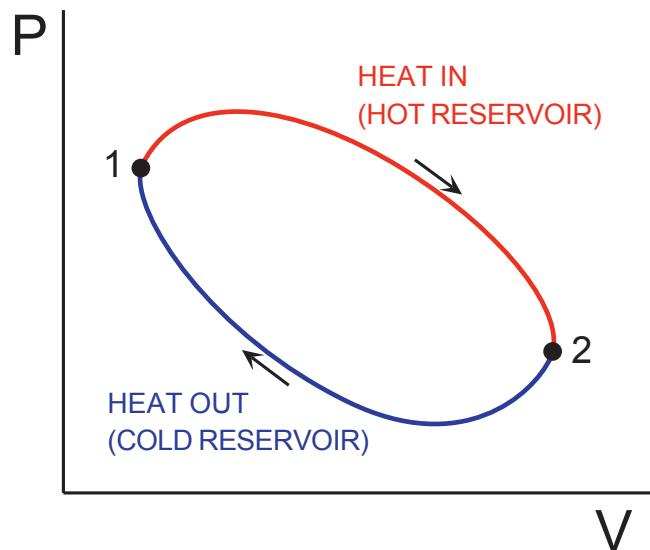
$$\begin{aligned}\Delta Q &\equiv \oint dQ \\ &= \underbrace{\int_1^2 dQ}_{\equiv |Q_H|} + \underbrace{\int_2^1 dQ}_{\equiv -|Q_C|}\end{aligned}$$
