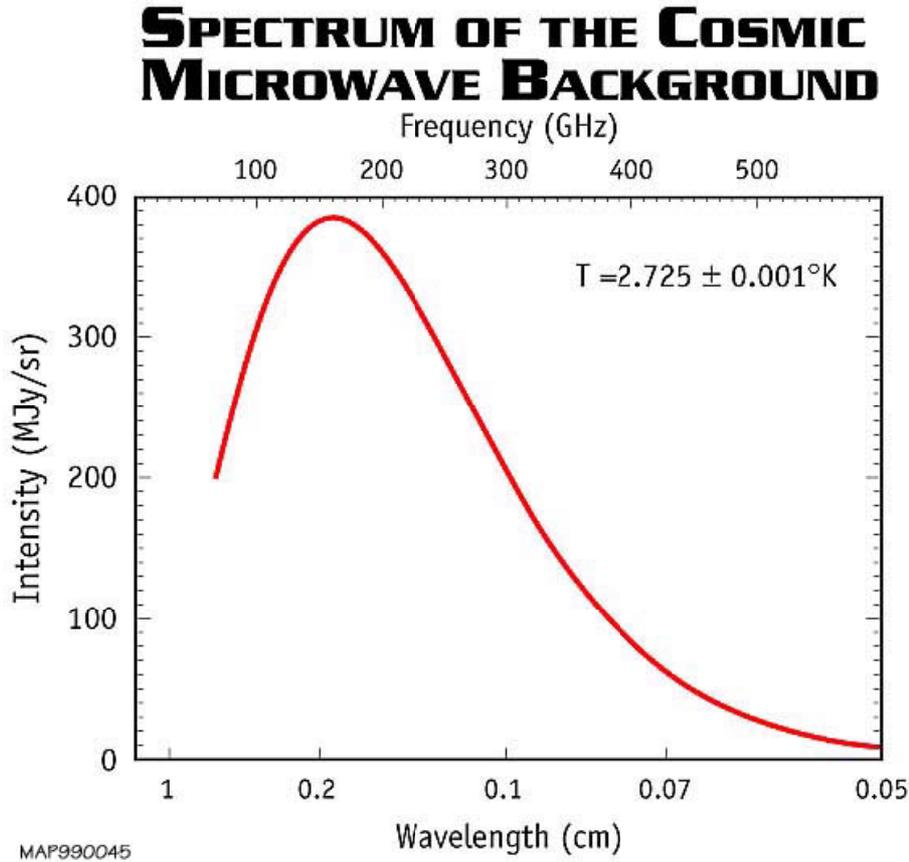
Figure 8: Spectrum of the cosmic microwave background radiation measured in the 1990s by the FIRAS instrument aboard the COBE satellite. (From the WMAP website.)
