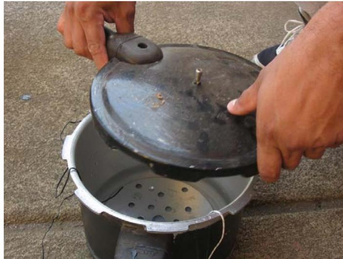
**Figure 2: Surface Temperature Sensors Inside Pressure Vessel.** The white surface temperature sensor was immersed in water, while the black surface temperature sensor was suspended in the air to measure the vapor temperature. Temperature sensors were secured in place through friction with the pressure vessel lid.
