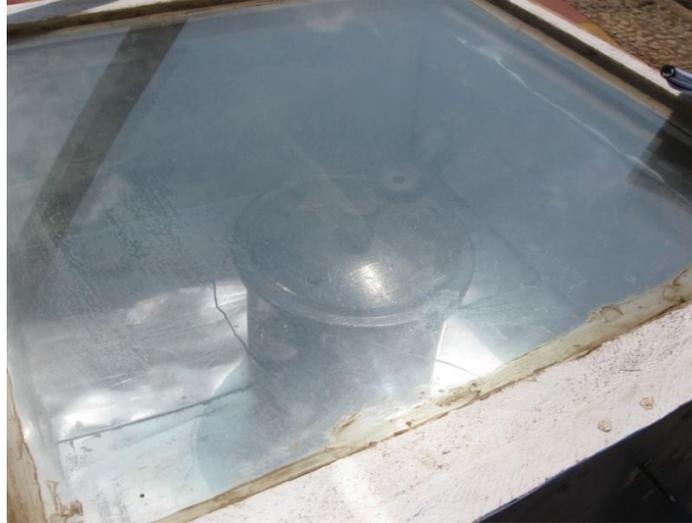
**Figure 3: Pressure Vessel with Temperature Sensors Inside Solar Oven.** The pressure vessel, with its surface temperature sensors, was placed in the center of the solar oven. Wires to the surface temperature sensors were passed through the door of the oven, which was then closed. In the back left corner of the solar oven, several inches from the pressure vessel, was an ACURITE brand oven thermometer used to measure the oven's interior air temperature.
