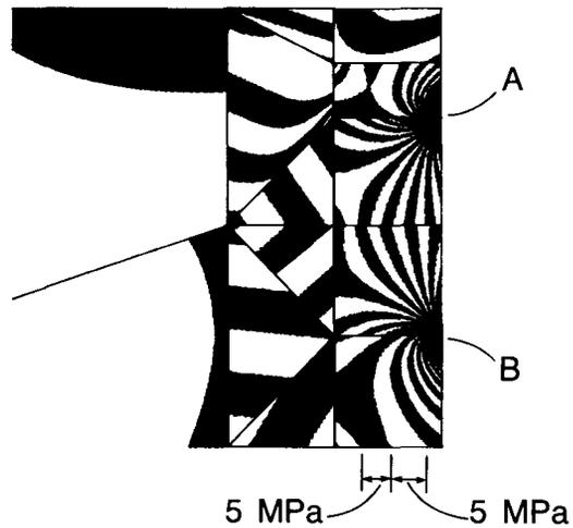
Based on the pressure band plot, we conclude that the mesh is too coarse for accurate stress prediction.
