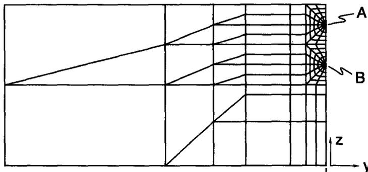
All elements are either 6- or 8-node isoparametric elements.
