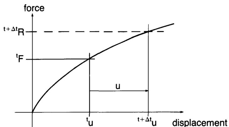
All we have done so far is to write the principle of virtual work in terms of  ${}^t u_i$  and  $u_i$ .
