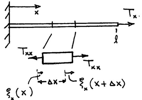
Prob. 7.14.1 Consider the relative deformations of material having the initial relative displacement  $\Delta\bar{r}$ , as shown in the sketch.
