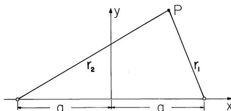
**Fig. 4.6.4** Definition of coordinates for finding field from line charges of opposite sign at  $x = \pm a$ . The displacement vectors are two dimensional and hence in the  $x - y$  plane.
