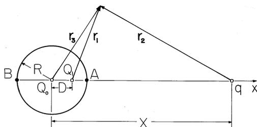
**Fig. 4.6.7** Cross-section of spherical electrode having radius  $R$  and center at the origin of  $x$  axis, showing charge  $q$  at  $x = X$ . Charge  $Q_1$  at  $x = D$  makes spherical surface an equipotential, while  $Q_o$  at origin makes the net charge on the sphere zero without disturbing the equipotential condition.
