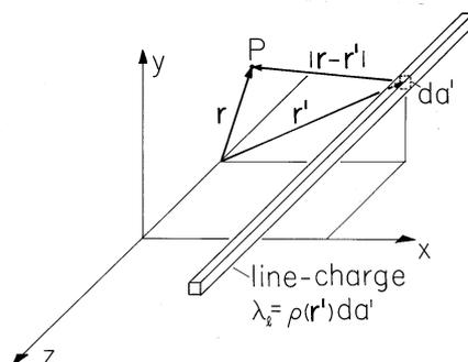
**Fig. 4.5.7** For two-dimensional charge distributions, the elementary charge takes the form of a line charge of infinite length. The observer and source position vectors,  $\mathbf{r}$  and  $\mathbf{r}'$ , are two-dimensional vectors.
