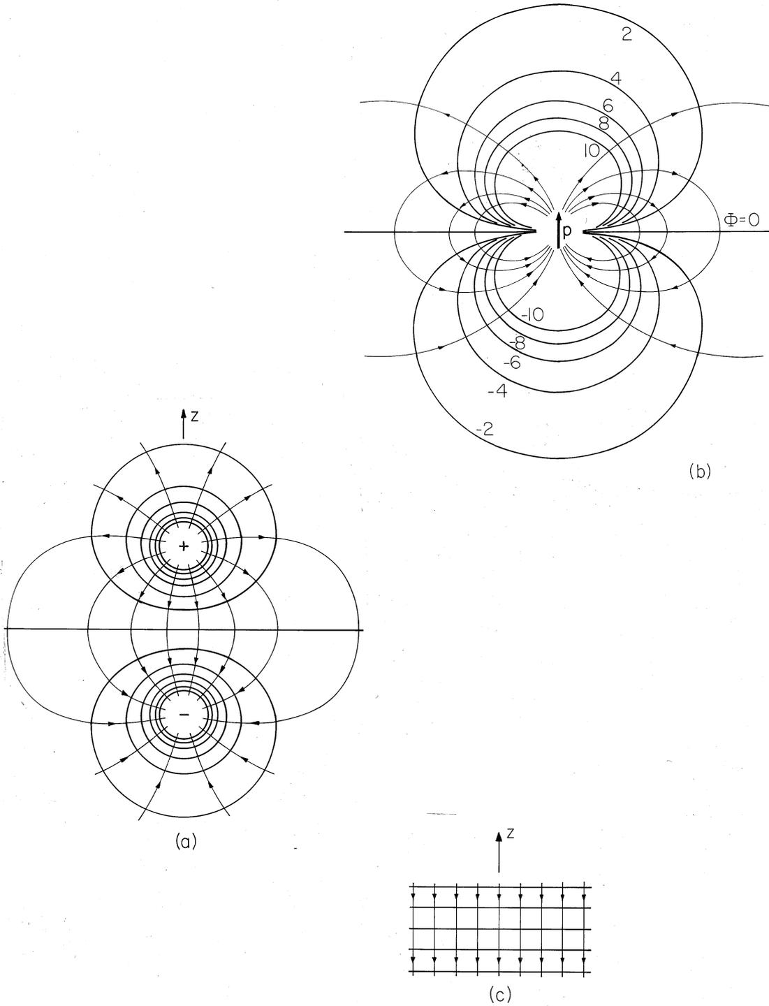
**Fig. 4.4.2** (a) Cross-section of equipotentials and lines of electric field intensity for the two charges of Fig. 4.4.1. (b) Limit in which pair of charges form a dipole at the origin. (c) Limit of charges at infinity.
