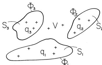
**Fig. 4.6.1** Once the superposition principle has been used to determine the potential, the field in a volume  $V$  confined by equipotentials is just as well induced by perfectly conducting electrodes having the shapes and potentials of the equipotentials they replace.
