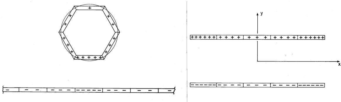
**Fig. 4.8.1** (a) Surface of circular cylinder over a ground plane broken into planar segments, each having a uniform surface charge density. (b) Special case where boundaries are in planes  $y = \text{constant}$ .
