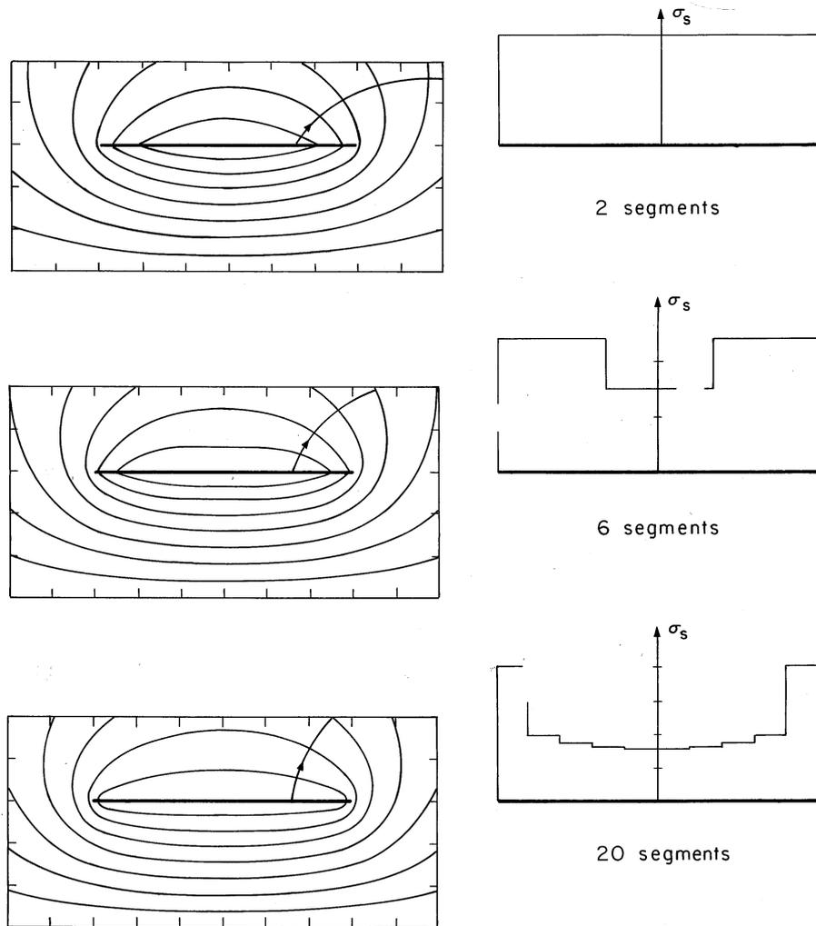
**Fig. 4.8.4** Potential distributions using 2, 6, and 20 sheets to approximate the fields of a plane parallel capacitor. Only the fields in the upper half-plane are shown. The distributions of surface charge density on the upper plate are shown to the right.
