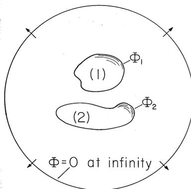
Fig. 4.6.2 Pair of electrodes used to define capacitance.
