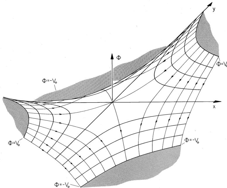
**Fig. 4.1.4** Two-dimensional potential of (18) and Fig. 4.1.3 represented in three dimensions. The vertical coordinate, the potential, is analogous to the vertical deflection of a taut membrane. The equipotentials are then contours of constant altitude on the membrane surface.
