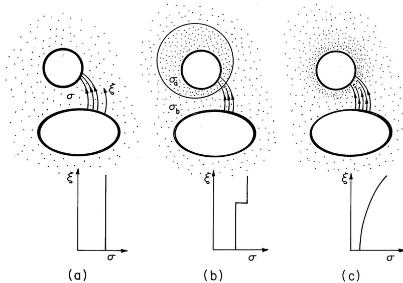
**Fig. 7.2.3** Typical configurations involving a conducting material and perfectly conducting electrodes. (a) Region of interest is filled by material having uniform conductivity. (b) Region composed of different materials, each having uniform conductivity. Conductivity is discontinuous at interfaces. (c) Conductivity is smoothly varying.
