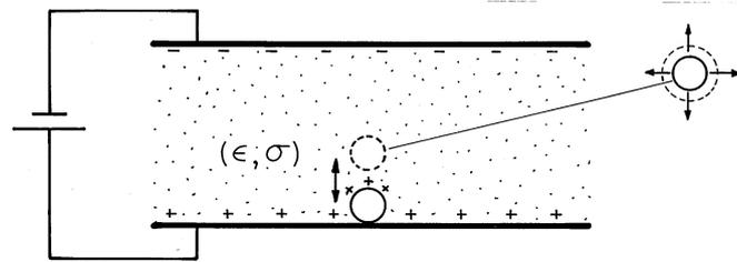
**Fig. 7.7.2** The region between plane parallel electrodes is filled by a semi-insulating liquid. With the application of a constant potential difference, a metal particle resting on the lower plate makes upward excursions into the fluid. [See footnote 1.]
