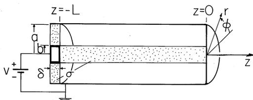
**Fig. 7.5.3** Circular cylindrical conductor surrounded by coaxial perfectly conducting “can” that is connected to the right end by a perfectly conducting “short” in the plane  $z = 0$ . The left end is at potential  $v$  relative to right end and surrounding wall and is connected to that wall at  $z = -L$  by a washer-shaped resistive material.
