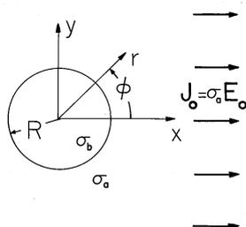
**Fig. 7.5.1** Conducting circular rod is immersed in a conducting material supporting a current density that would be uniform in the absence of the rod.
