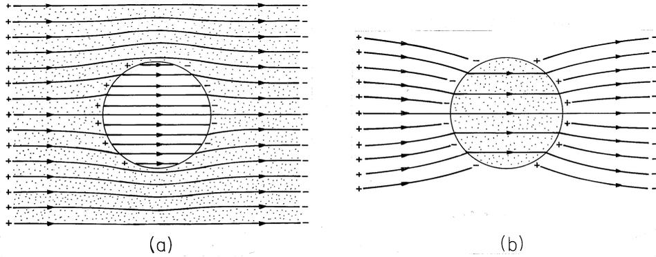
**Fig. 7.5.6** Distributions of *electric field* intensity around conducting rod immersed in conducting medium: (a)  $\sigma_a \gg \sigma_b$ ; (b)  $\sigma_b \gg \sigma_a$ . Compare these to distributions of *current density* shown in Fig. 7.5.2.
