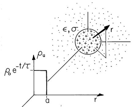
**Fig. 7.7.1** Within a material having uniform conductivity and permittivity, initially there is a uniform charge density  $\rho_u$  in a spherical region, having radius  $a$ . In the surrounding region the charge density is given to be initially zero and found to be always zero. Within the spherical region, the charge density is found to decay exponentially while retaining its uniform distribution.
