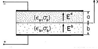
Fig. 7.9.3 Maxwell's capacitor.
