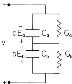
Fig. 7.9.5 Maxwell's capacitor, Fig. 7.9.3, is exactly equivalent to the circuit shown.
