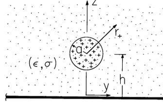
**Fig. 7.9.1** Infinite half-space of material having uniform conductivity and permittivity is bounded from below by a perfectly conducting plate. When  $t = 0$ , there is a uniform charge density in a spherical region.
