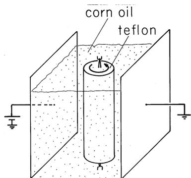
**Fig. 7.5.7** Rotor of insulating material is immersed in somewhat conducting corn oil. Plane parallel electrodes are used to impose constant electric field, so from the top, the distribution of electric field should be that of Fig. 7.5.6a, at least until the rotor begins to rotate spontaneously in either direction.
