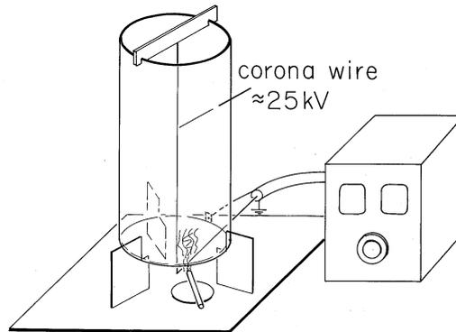
**Fig. 7.7.5** Electrostatic precipitator consisting of fine wire at high voltage relative to surrounding conducting transparent coaxial cylinder. Ions created in corona discharge in the immediate vicinity of the wire follow field lines toward outer wall, some terminating on smoke particles. Once charged by the mechanism described in Example 7.7.2, the smoke particles are precipitated on the outer wall.
