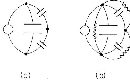
**Fig. 7.0.1** EQS distributions of potential and current density are analogous to those of voltage and current in a network of resistors and capacitors. (a) Systems of perfect dielectrics and perfect conductors are analogous to capacitive networks. (b) Conduction effects considered in this chapter are analogous to those introduced by adding resistors to the network.
