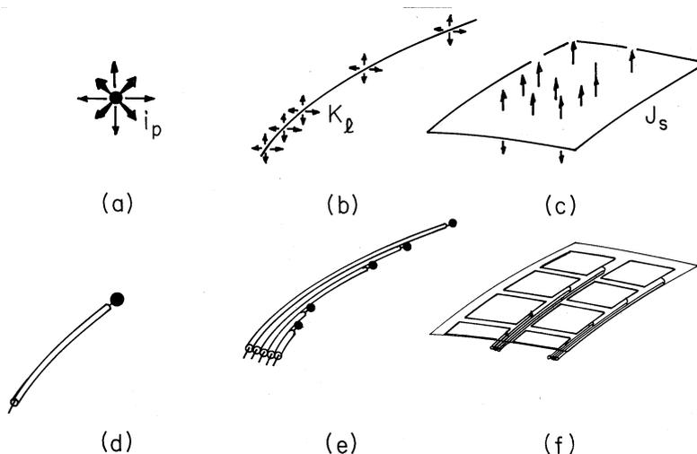
**Fig. 7.3.1** Singular current source distributions represented conceptually by the top row, suggesting how these might be realized physically by the bottom row by electrodes fed through insulated wires.
