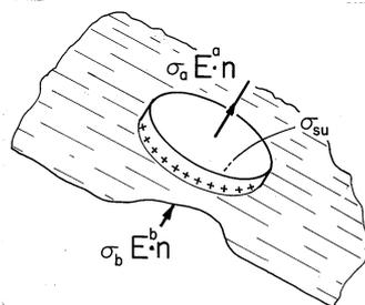
**Fig. 7.9.2** Incremental volume for writing charge conservation boundary condition.
