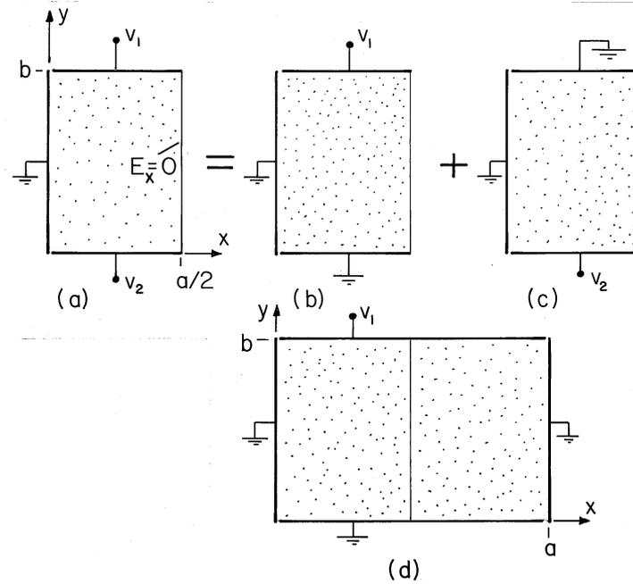
**Fig. 7.4.1** (a) Two terminal pairs attached to conducting material having one wall at zero potential and another that is insulating. (b) Field solution is broken into part due to potential  $v_1$  and (c) potential  $v_2$ . (d) The boundary condition at the insulating wall is satisfied by using the symmetry of an equivalent problem with all of the walls constrained in potential.
