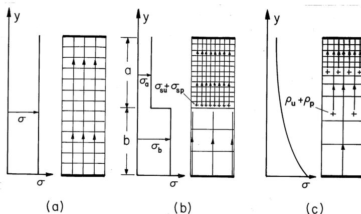
**Fig. 7.2.5** Conductivity, potential, charge density, and field distributions in special cases for the configuration of Fig. 7.2.4. (a) Uniform conductivity. (b) Layers of uniform but different conductivities. (c) Exponentially varying conductivity.
