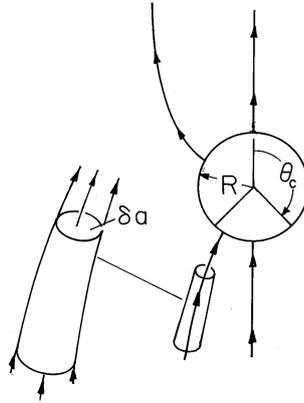
**Fig. 7.7.3** Particle immersed in an initially uniform electric field is charged by unipolar current of positive ions following field lines to its surface. As the particle charges, the “window” over which it can collect ions becomes closed.
