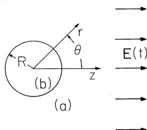
**Fig. 7.9.6** A spherical material with conductivity  $\sigma_b$  and permittivity  $\epsilon_b$  is surrounded by a material with conductivity and permittivity  $(\sigma_a, \epsilon_a)$ . An electric field  $E(t)$  that is uniform far from the sphere is applied.
